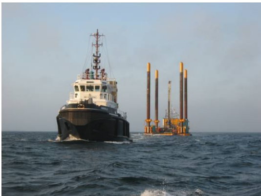
Towing jack-up barge 'Octopus' to installation site.
