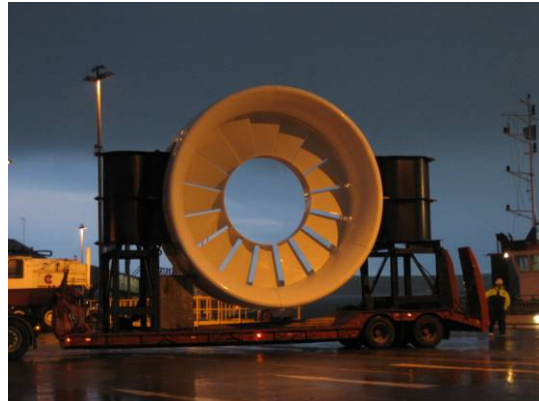
Transporting Open-Centre Turbine
